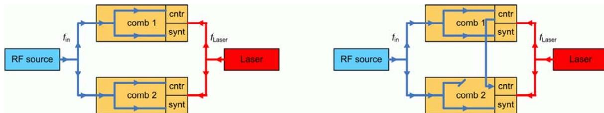
Figure 1: Schematic setup for a comb-comb comparison. Left setup without synchronisation, right with counter synchronisation. *cntr*: counter, *synt*: RF-synthesizer. RF signals are denoted by blue lines and  $f_{in}$ , optical signals by red lines and  $f_{Laser}$ .
