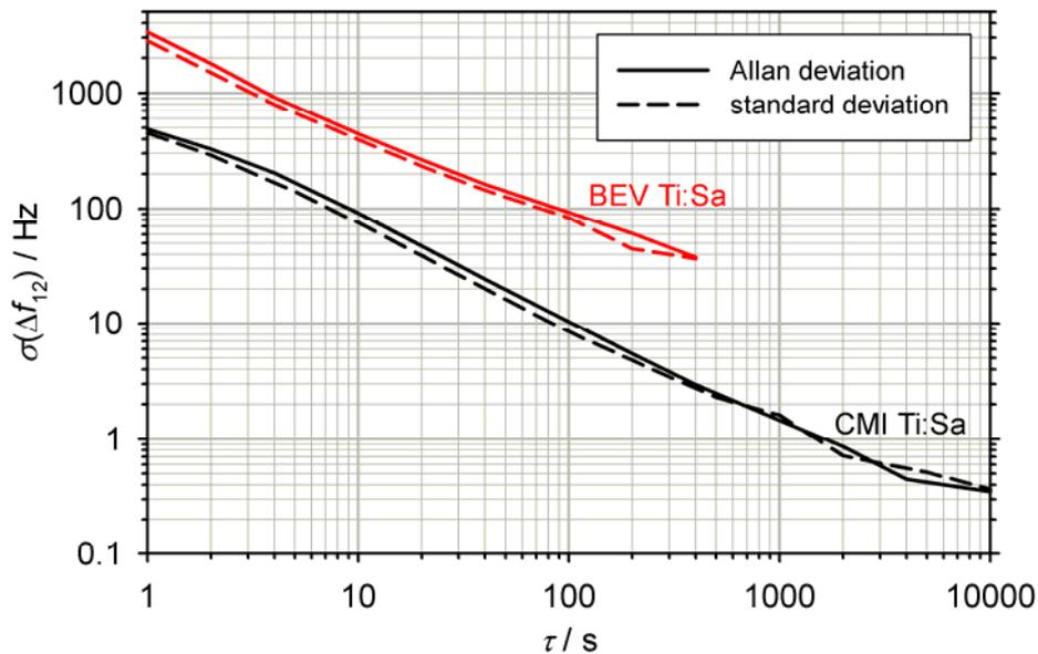
Figure 3: Allan standard deviation (solid lines) and sample standard deviation (dashed lines) for the frequency difference between BEV fibre comb and the two other combs considered.
