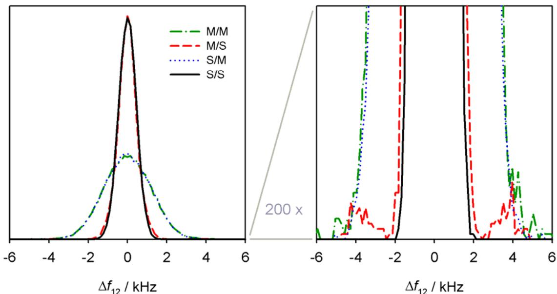
Figure 4: Histograms for 1 second samples of  $\Delta f_{12}$  when the repetition frequency is measured (M) or servo controlled (S). First comb is CMI Ti:Sa, second BEV fibre, respectively. In the right hand side of the picture the ordinate is enlarged by 200 times to demonstrate small differences in the side wings.
